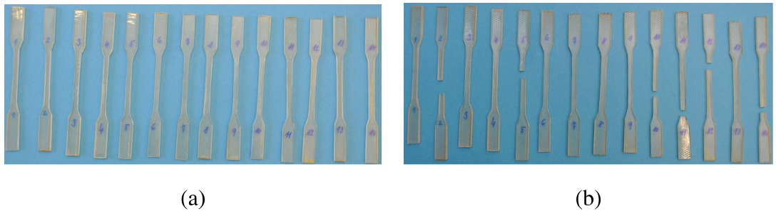
Figure 4.2: Specimens used in tensile and creep tests: a) Prior to testing, b) After testing
