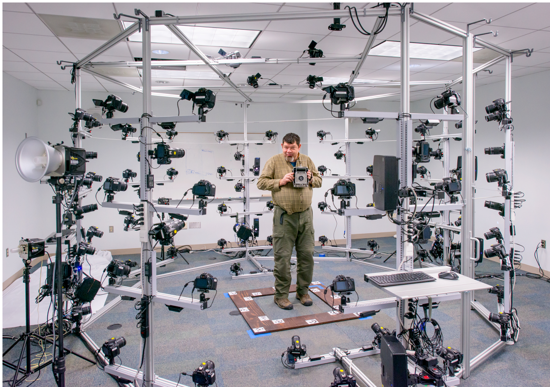
■ Figure 2.6 Multi-camera system at University of Maryland [21]
