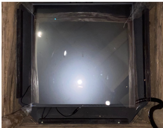
Figure 3.27: Visible reflection on display plastic protection
