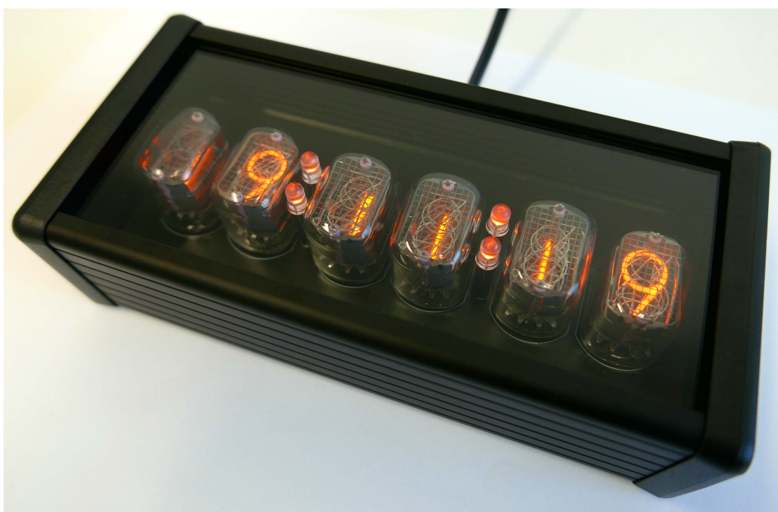
■ Figure 5.1 A fully-assembled nixie clock device. (© Matěj Bartík)
