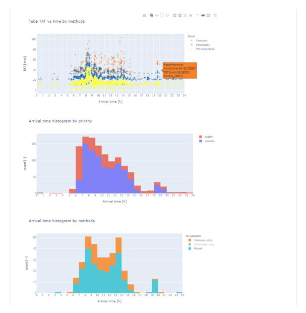
Figure 8: Samples - pre-analytical and method result time, arrival time histograms by priority and method types
