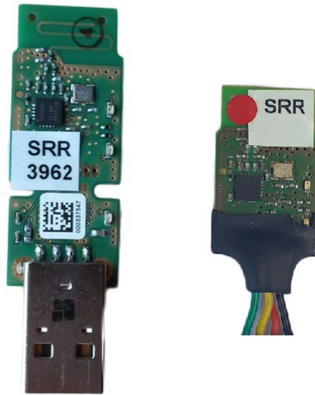
Figure 3.5: The inner piece of SPORTident SRR dongle
