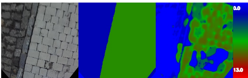
Figure 9.5: Example of friction map on cobbles tiled pavement (Original image -> Manual annotation -> Model prediction -> Value bar)
