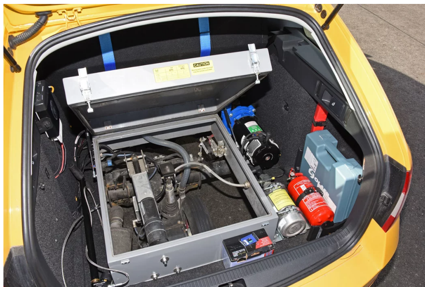
Figure 3.1: Trunk of the car measuring surface friction on Prague airport [8]
