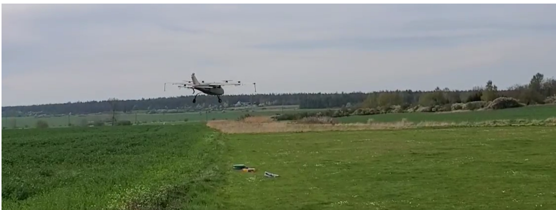
Figure 8.2. Drone during yaw control tests.
