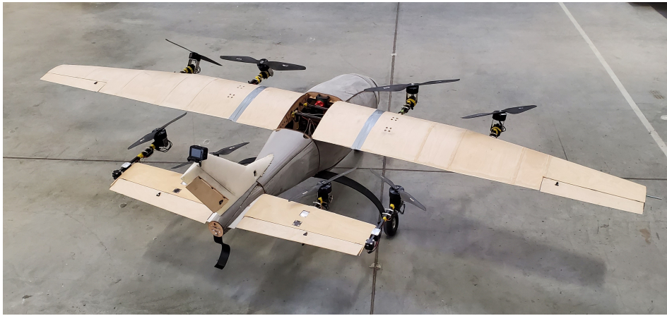
Figure 6.1. The eVTOL drone, designed by Ing. Filip Tomáš, that has been used for verification of the control algorithms.
