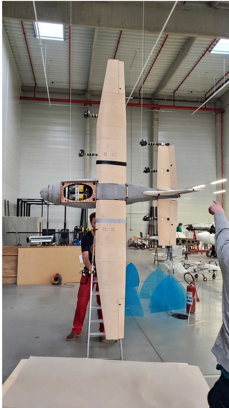
Figure B.1. Measurement of the drone's moments of inertia using the pendulum method.
