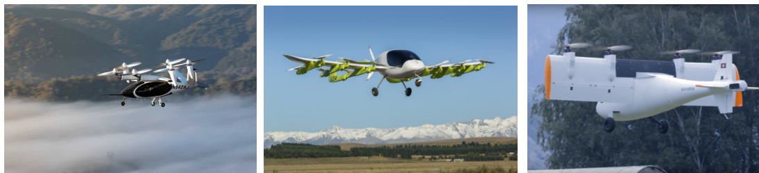
Figure 1.2. Examples of current civil VTOL aircraft prototypes, Joby tilt-rotor on the left [3], Wisk lift and thrust in center [4] and Dufour tilt-wing on the right [5].
