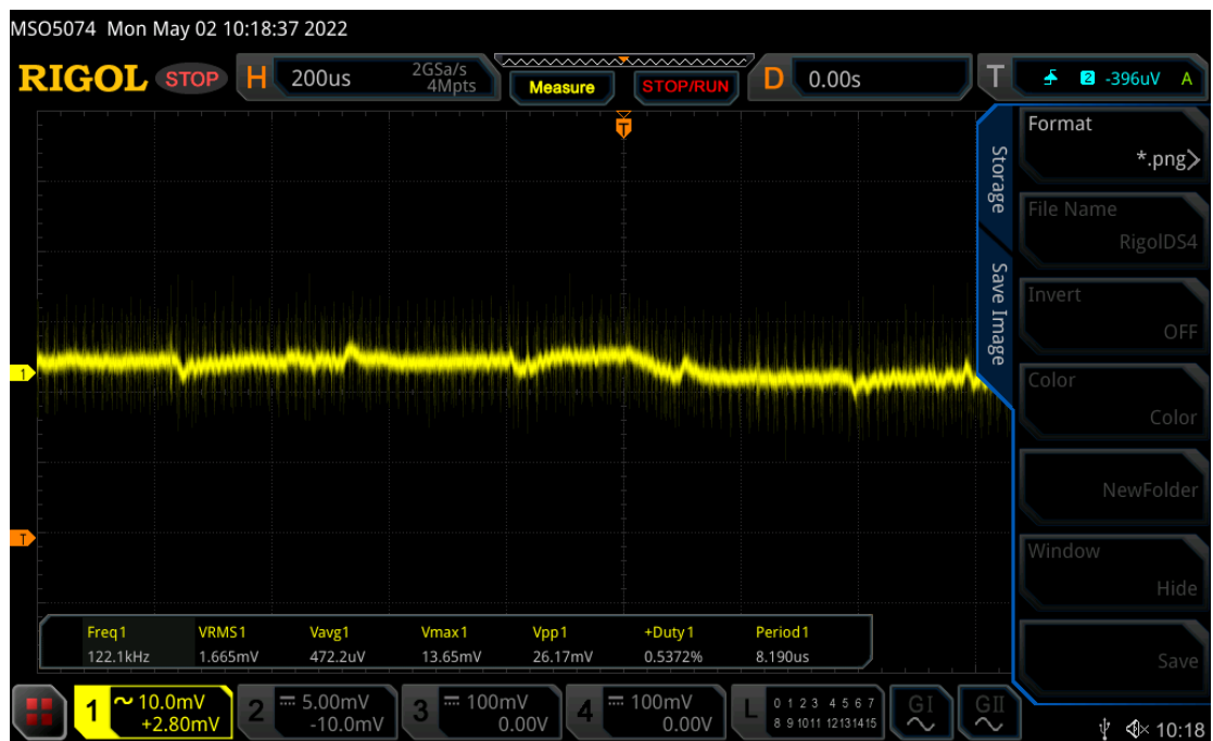
Figure 7.3. +3V3 supply rail AC oscillogram, measured between the sequencer daughter-board TC1015 regulator output and ground pin. The modules were operated in standard mode during measurement. The STM32F7308 Discovery Kit was powered by the STLink USB connector connected to a battery-powered notebook USB port.
