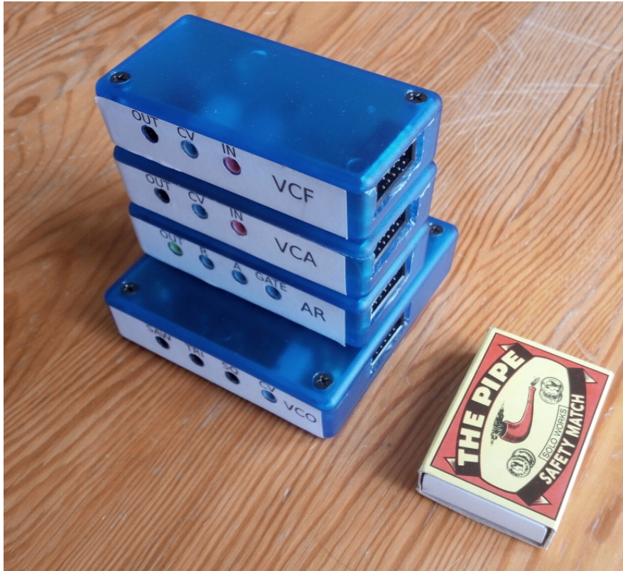
Figure 4.1. Photo of all modules that are in enclosures. A standard size matchbox is included for size reference.
