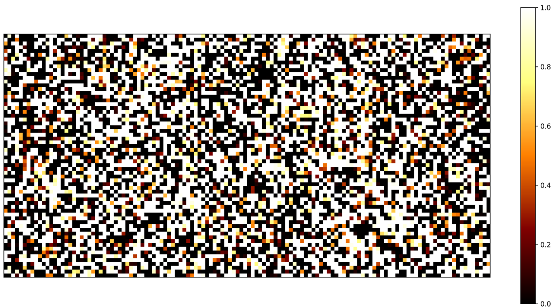
■ Figure 2.3 Average startup values of individual SRAM cells over 1000 measurements. White bits are stable '1', black bits are stable '0' and the rest are unstable bits with varying amounts of bias (according to the color bar on the right). Cells with an average value of 0.5 are the least stable. The data was obtained from ESP32 number 12 at 20°C.
