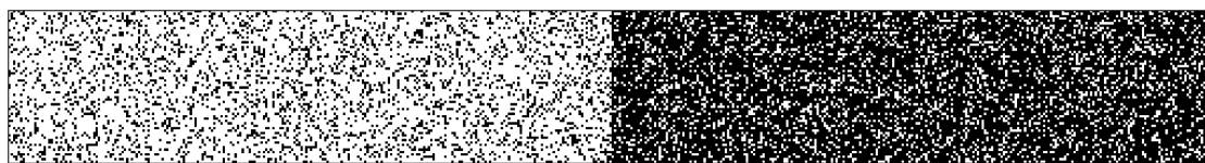
■ Figure 4.8 Visualization of PUF response from MCU 16 in a 512 \times 64 bit grid (RTC SRAM method)
