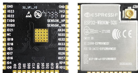
■ Figure 3.1 The ESP32-WROOM-32U module back and front image [46]
