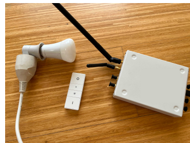
Fig. 3. Testbed consisting of SDR Ettus USRP B210, lightbulb Philips LWB004 with firmware version 5.127.1.26420 and Philips 324131137411 remote utilised in testing of our tool zigtoucher used for security analysis of ZigBee Touchlink
