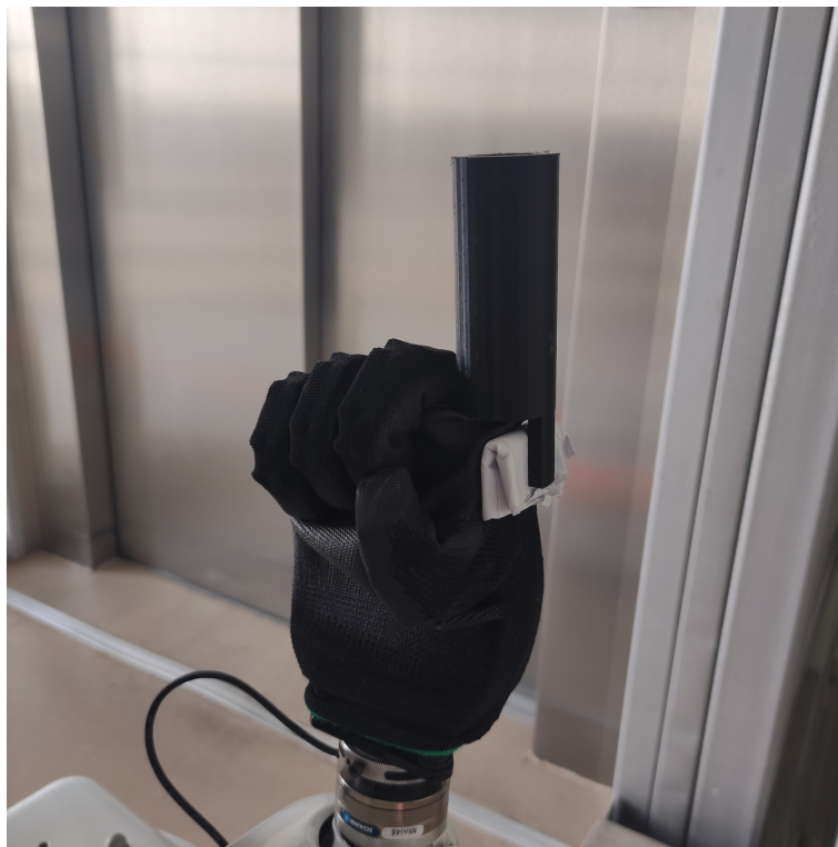
Figure 5.1. TIAGo's hand equipped to press buttons.
