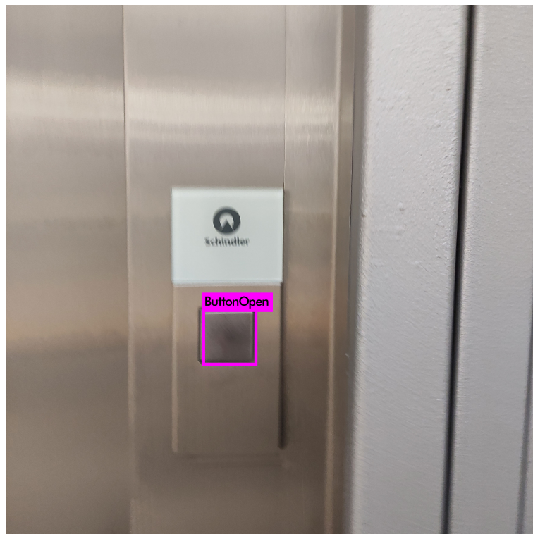
Figure 5.2. YOLO detection of outside elevator button.
