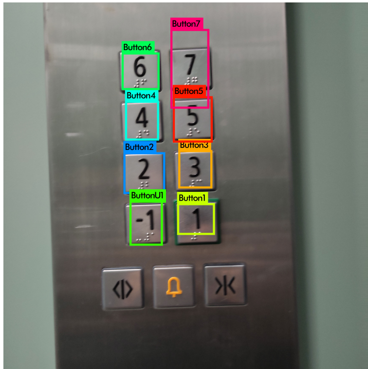
Figure 5.4. YOLO detection of the buttons inside of the elevator after taking their most probable position.
