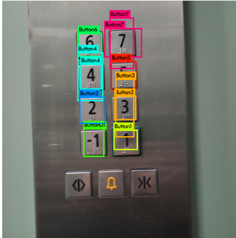
Figure 5.3. YOLO detection of the buttons inside of the elevator.
