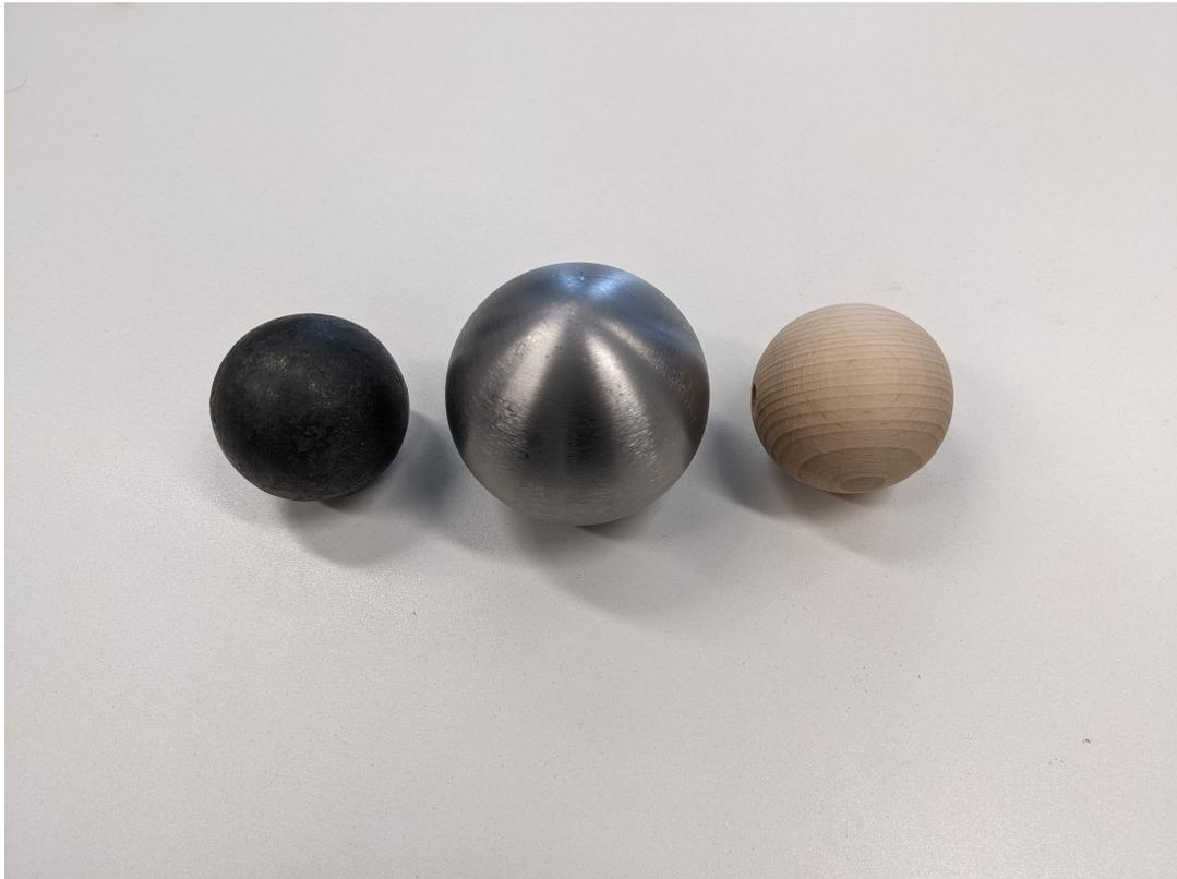
■ **Figure 3.2** Wrought iron sphere, aluminium sphere, and wooden sphere with a radius of 30 mm, 40 mm, and 30 mm, respectively
