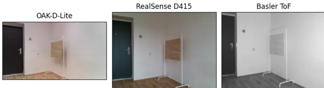
■ **Figure 4.6** Wooden board captured from 3000 mm under a 60-degree incidence angle.
