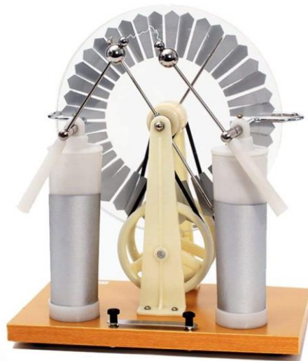
Figure 2.4: Wimshurst electrostatic generator adapted from [10]
