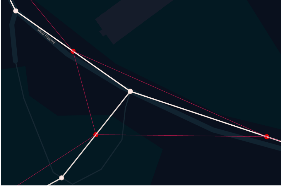
Figure 5.9: The edge based representation (red) of a junction in the original graph (white).
