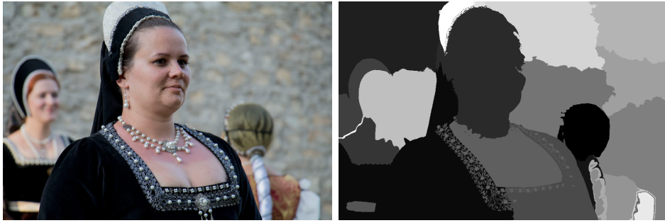
Figure 4.2: Comparison of source image and the resulting clusters after application of k-means algorithm
