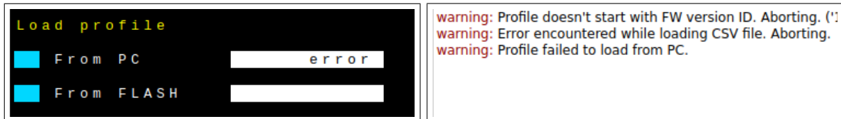
Figure 30: Load profile menu after an error occurred (left), corresponding error message (right)
