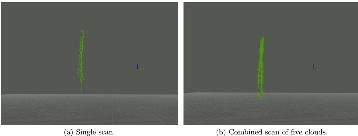
Figure 5.3: Input point cloud for ICP Fig. 5.3a shows single cloud, Fig. 5.3b shows combination of 5 most recent scans.
