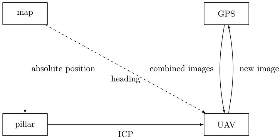
Figure 5.4: Diagram of how the absolute position of the UAV is obtained.
