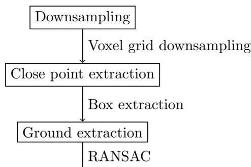
Figure 2.2: Diagram of dataflow in filter node.
