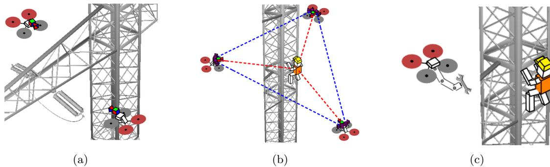
Figure 1.1: Visualization of possible usage of UAVs in power tower inspection task. Inspection of parts of the power tower Fig. 1.1a. Monitoring the safety of the workers Fig. 1.1b. Delivery of the equipment Fig. 1.1c. Those images were taken from article [1].
