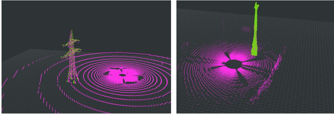
(a) Alignment of measured lidar scan and model in simulation.
