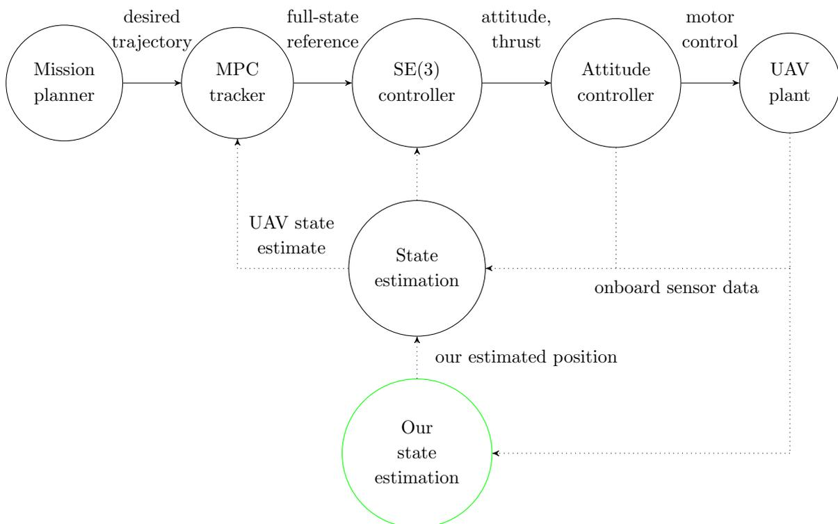
Figure 8.1: Diagram showing integration of our system into current architecture.
