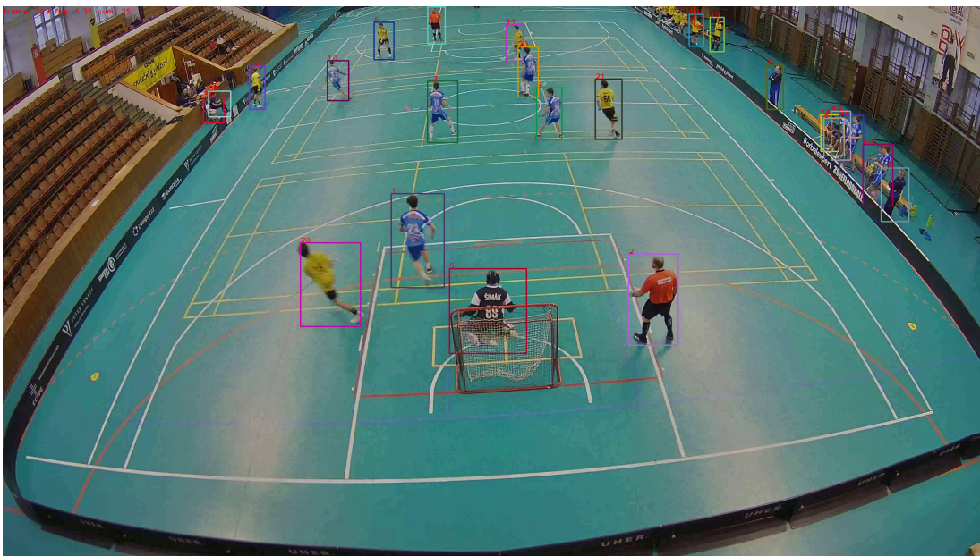
Figure 3.3. Example output of the single-camera detector. Small numbers are identities assigned by ByteTrack.
