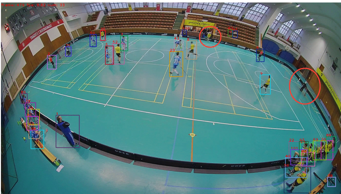
Figure 4.2. Example of false negative single-camera detections. The error emphasized in red circle.
