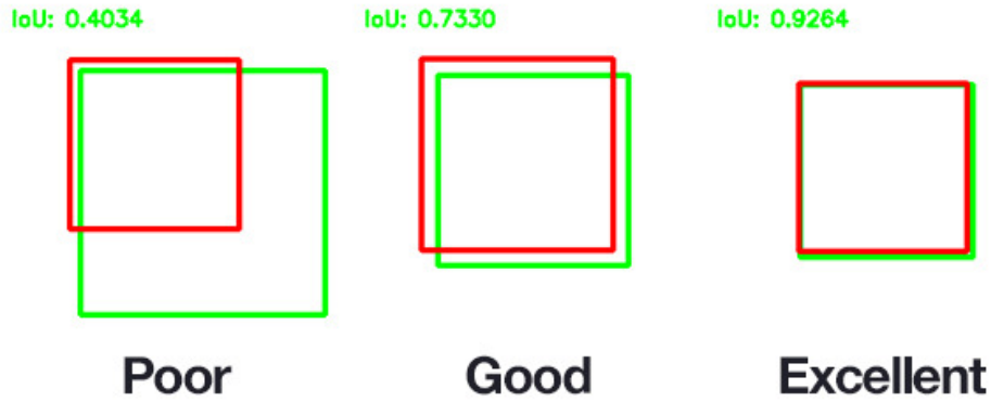
Figure 3.2: Examples of IOUs for different overlaps between GT and predicted box, source. [3]
