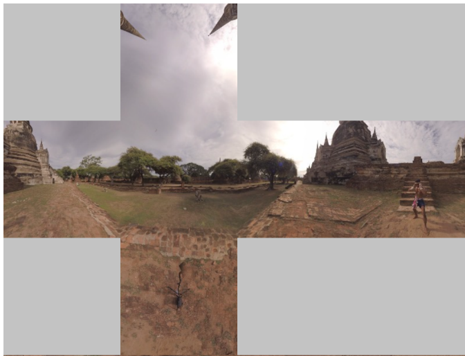
Figure 2.1: A Cubemap projection of omnidirectional footage, which is used by Unity.
