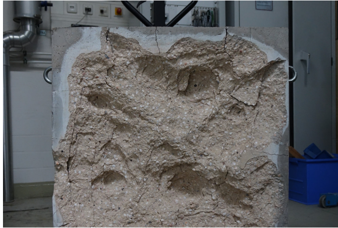
Figure 1.1.: Spalling damage to a concrete block after fire exposure. Image from experiments performed at the Federal Institute for Materials Research and Testing in Berlin.
