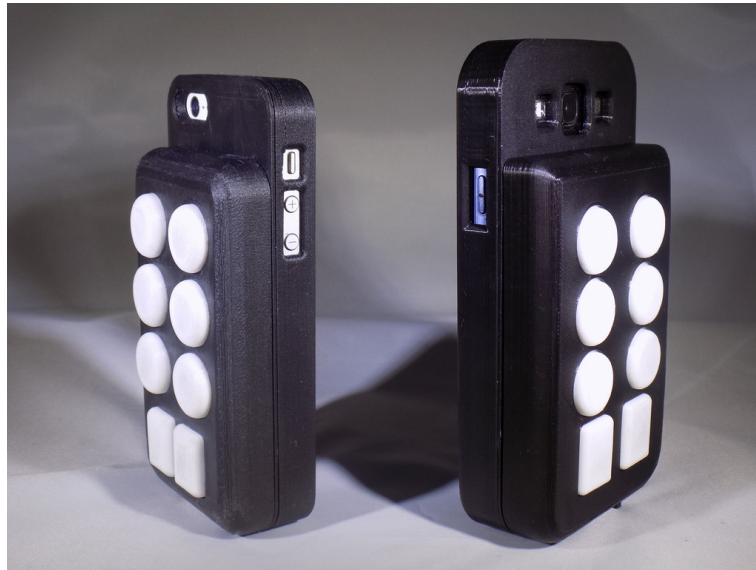
Figure 2.9. BrailleTooth cases, 3D printed prototypes, iPhone 5 case on the left, Samsung Galaxy S3 on the right. Source 8
