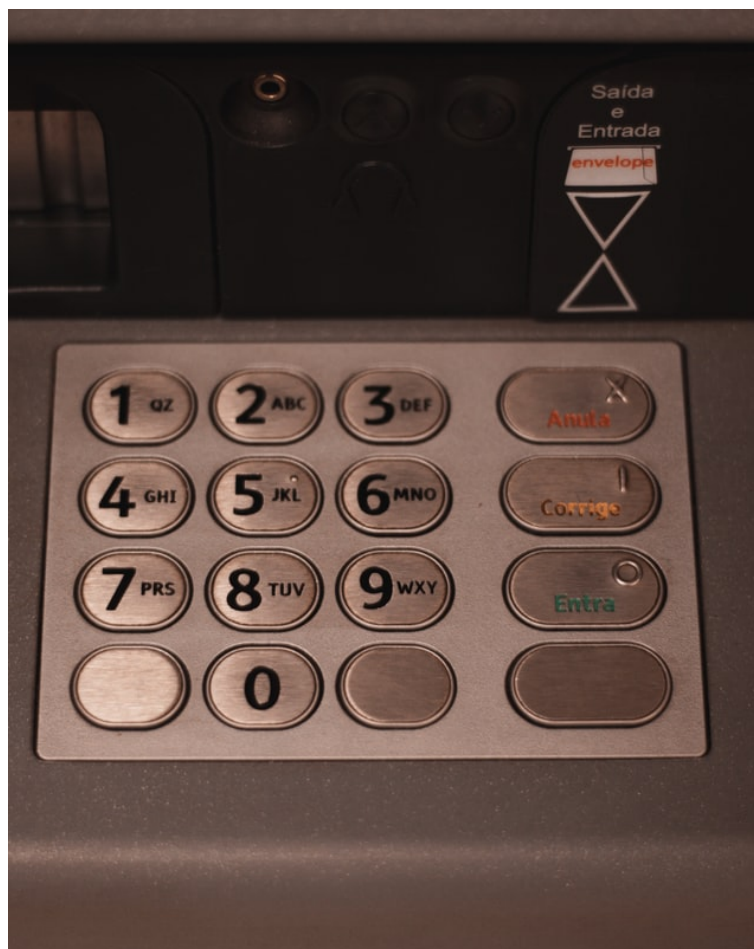
Figure 2.4. ATM Keypad with headphones jack and control buttons above. Source 3
