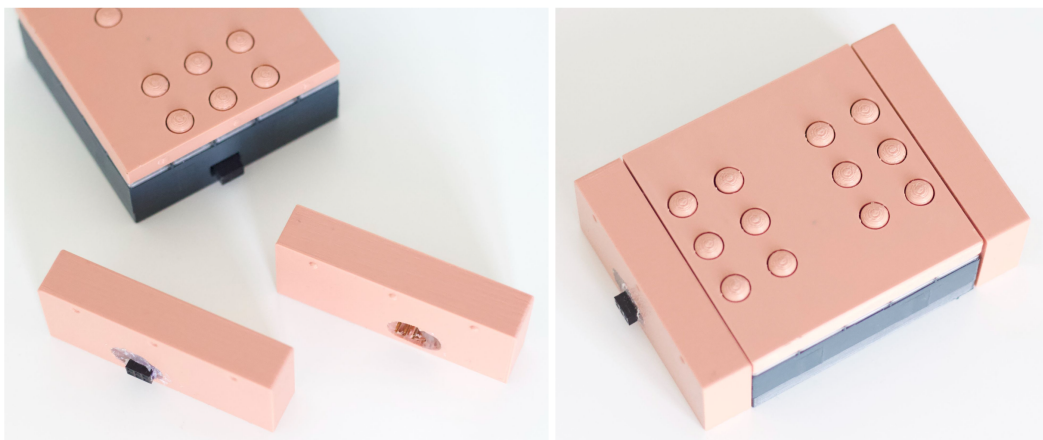
Figure 3.10. Detail of Spacer Blocks with the connectors on the left, assembled module with the spacer on the right.
