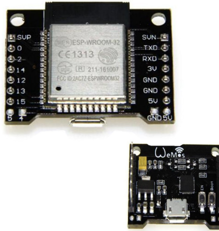
Figure 5.3: WeMos ESP-WROOM-32 , the ESP32 board used as the backbone of our prototype. Image from [15].
