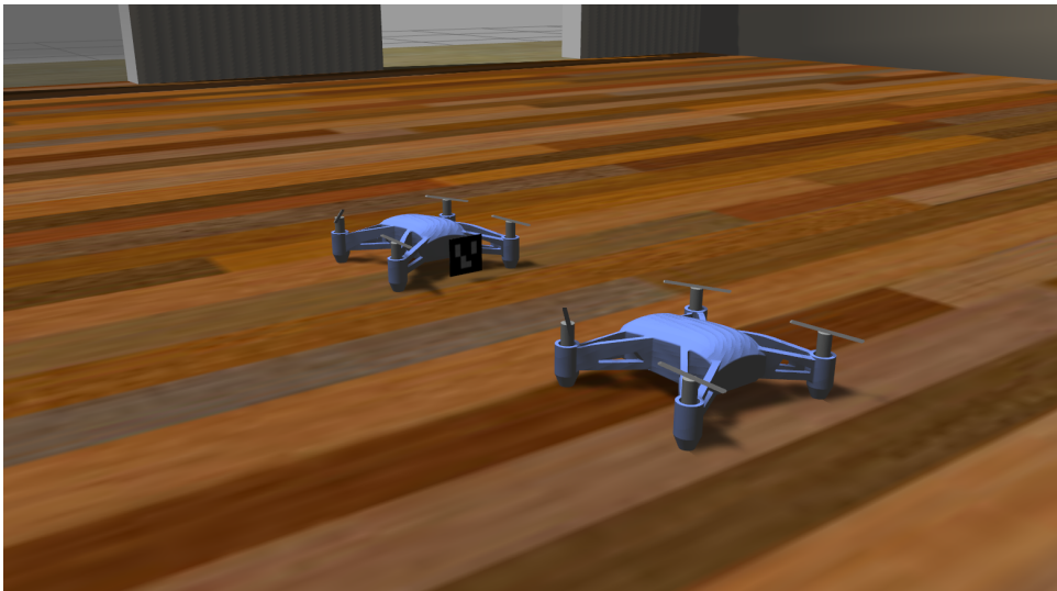
Figure 4.5: Complete simulation with two drones and ArUco marker attached to the leader.
