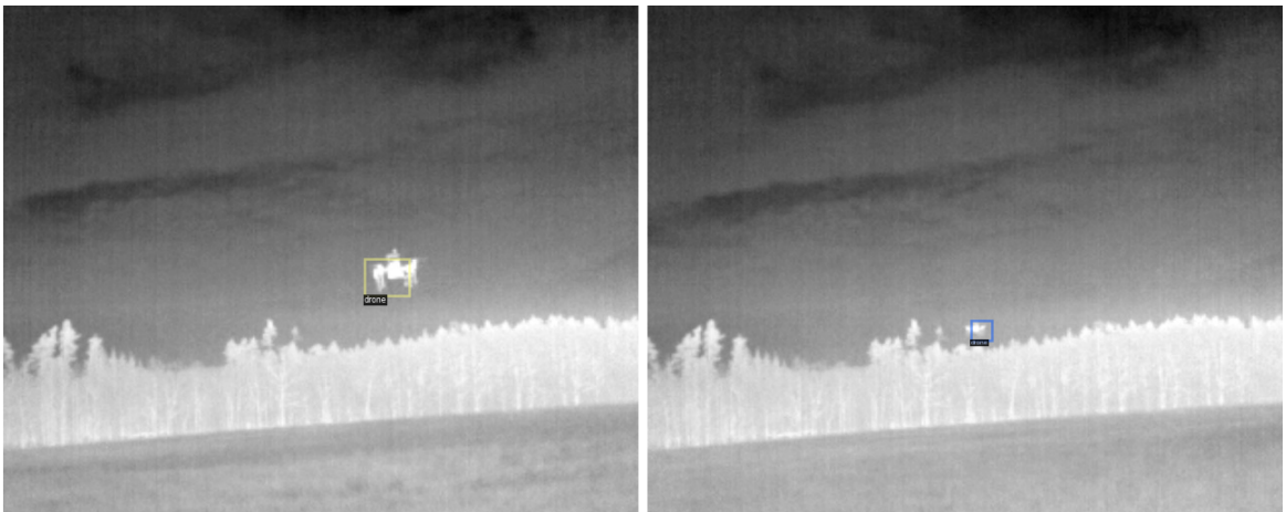
Figure 5.3: Examples of wrong ground truth boxes due to misaligned photos.
