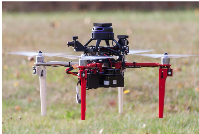
Figure 1.1: A flying quadcopter DJI F450 used for the experiments in this thesis 1 .
