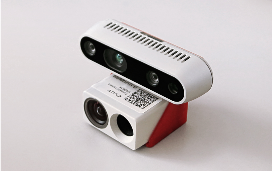
Figure 5.2: The RGB and thermal cameras mounted together.
