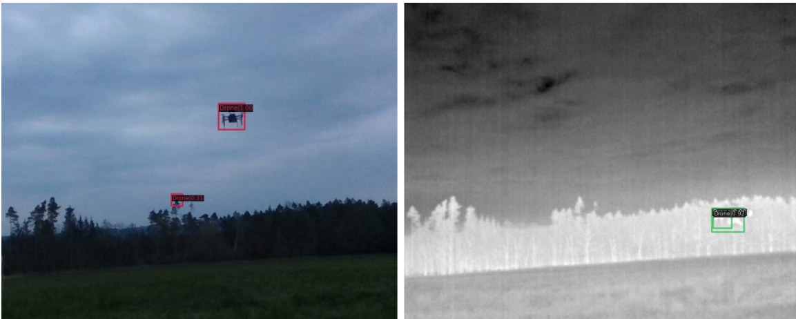
Figure 5.5: Examples of false positive results by the RGB (left) and the thermal (right) detectors in the evening dataset.
