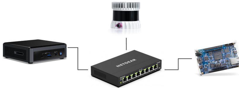
Figure 2: Schema of the switched network hosting the DE10-Nano board, Ouster OS0 LiDAR and Intel NUC. (Images from [25], [26], [27], [28].)
