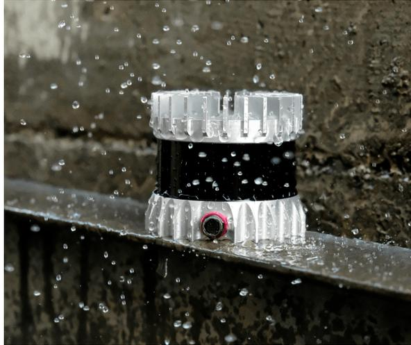
Figure 3: The used Ouster OS0 LiDAR. [29]
