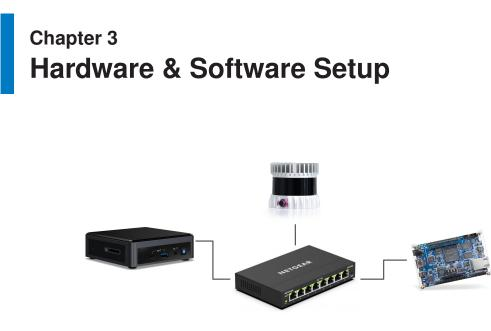
Figure 2: Schema of the switched network hosting the DE10-Nano board, Ouster OS0 LiDAR and Intel NUC. (Images from [25], [26], [27], [28].)
