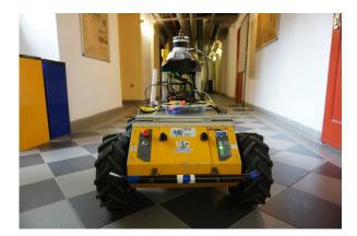
Figure 17: The Clearpath Husky A200<sup>TM</sup> robotic platform inside a hallway.
