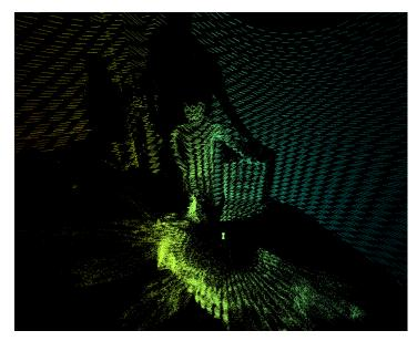
(a) Point cloud depicting a person standing near the LiDAR unit and leaning on a chair.
