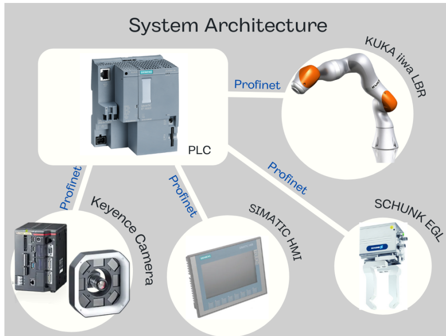
Figure 3.2: Final version of the system architecture.
