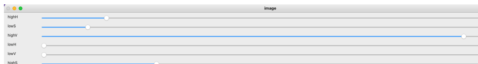
Figure 5.2: Slider bar for configuring filters in HSV domain.
