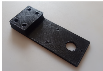
(b) : Magnetic rotary position sensor mounting 3D print
