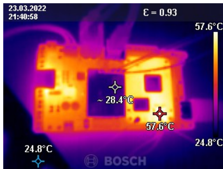
Figure 2.12: Thermal camera test
