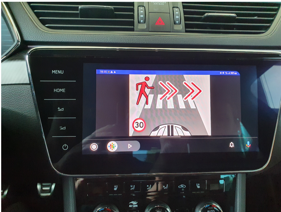
Figure 5.3: Red warning displayed on vehicle infotainment unit
