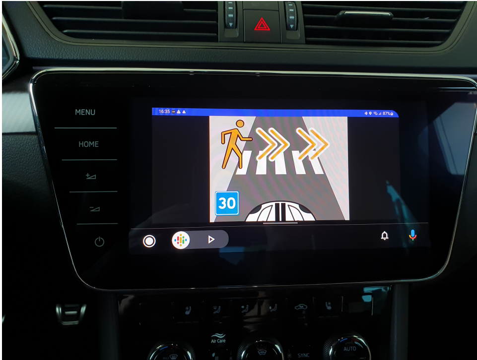
Figure 5.2: Orange warning displayed on vehicle infotainment unit
