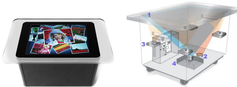
Figure 2.2: Microsoft PixelSense 1.0 (left) and its internal layout (right) 6 .
