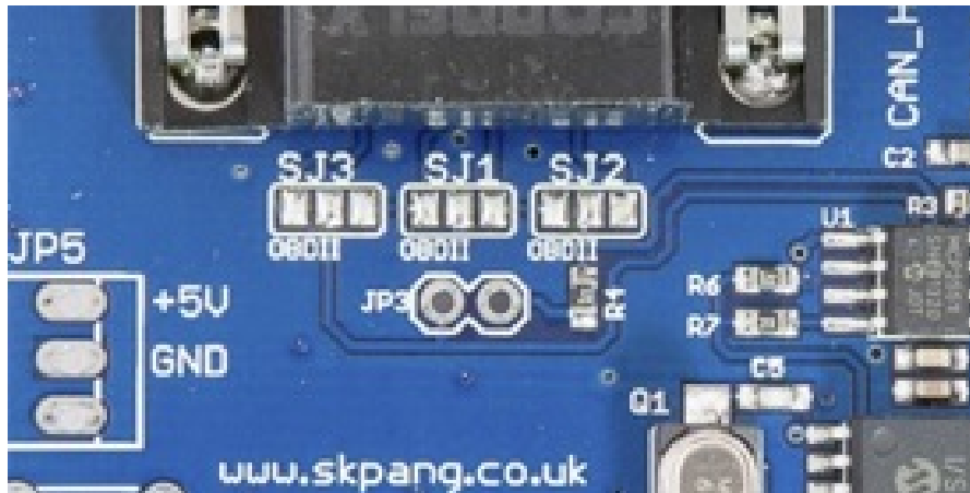
■ Figure 4.5 JP3 - 120 Ohm termination resistor [15]
