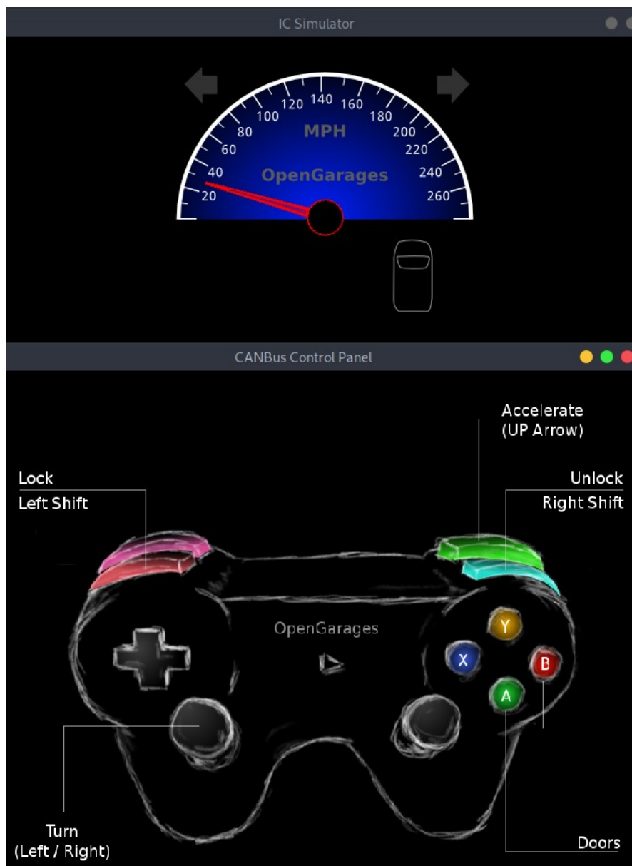
■ Figure 3.2 ICSim and controls interface
