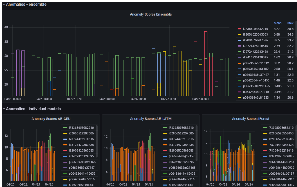
Figure 6.6: Grafana Dashboard containing anomaly scores from ensemble method ENS_3 and individual models for the time period of 7 days
