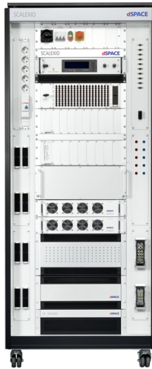
Figure 2.1: HiL simulator - taken from [6]
