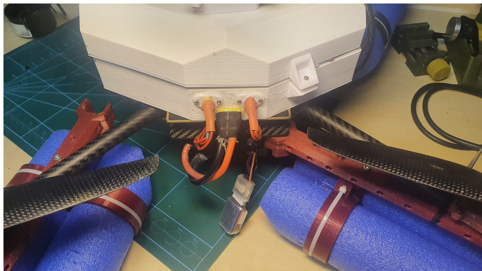
Figure 4.5: The newly implemented motor connection design.
