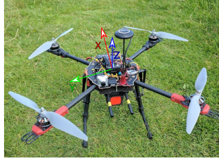
Figure 4.10: Visualisation of the x, y and z axes for the bifilar pendulum method.
