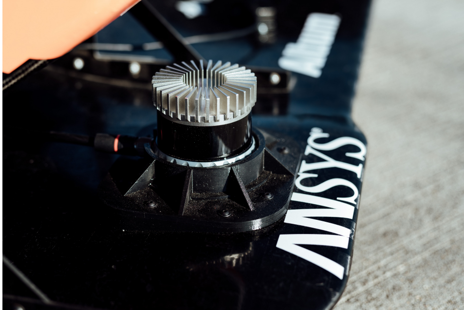
Fig. 10: LiDAR used on DV.01 - Ouster OS1-64 located on the front wing of the formula.
