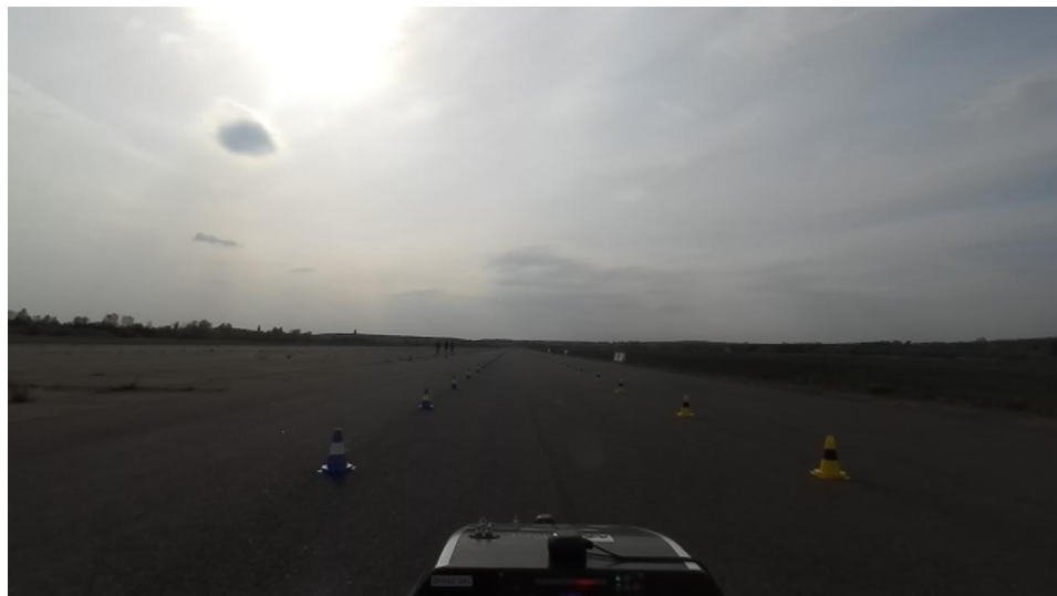
Fig. 6: Example of bad light conditions which are difficult for the camera to process. LiDAR
