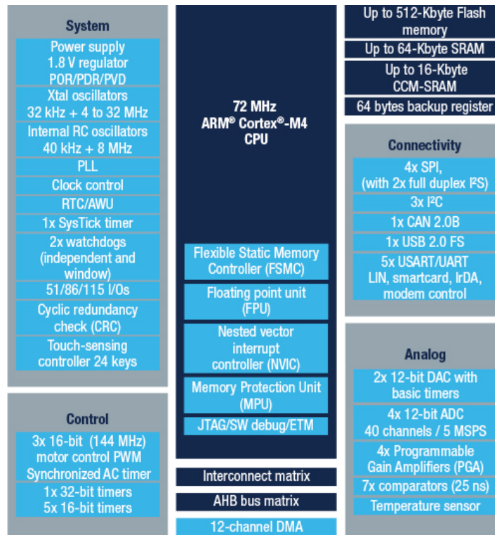
Figure 1: STM32F303 circuit diagram [6]
