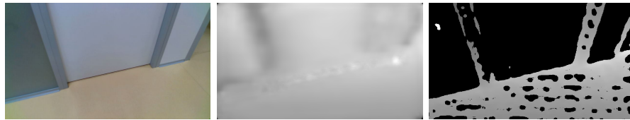
(b) : Example image, dense depth, and the ground truth, where ground truth is missing for a large part of the image
