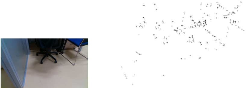
(b) : RGB Image from the robot and Sparse depth image from ORB SLAM
