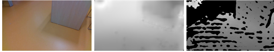
(a) : Image, predicted dense depth, and the ground truth depth
