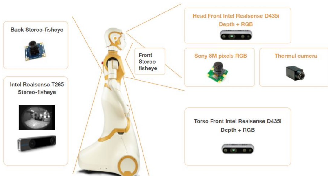
Figure 6.1: ARI Cameras Configuration. The Torso Front camera, an Intel Realsense D435i is used with ORB SLAM
