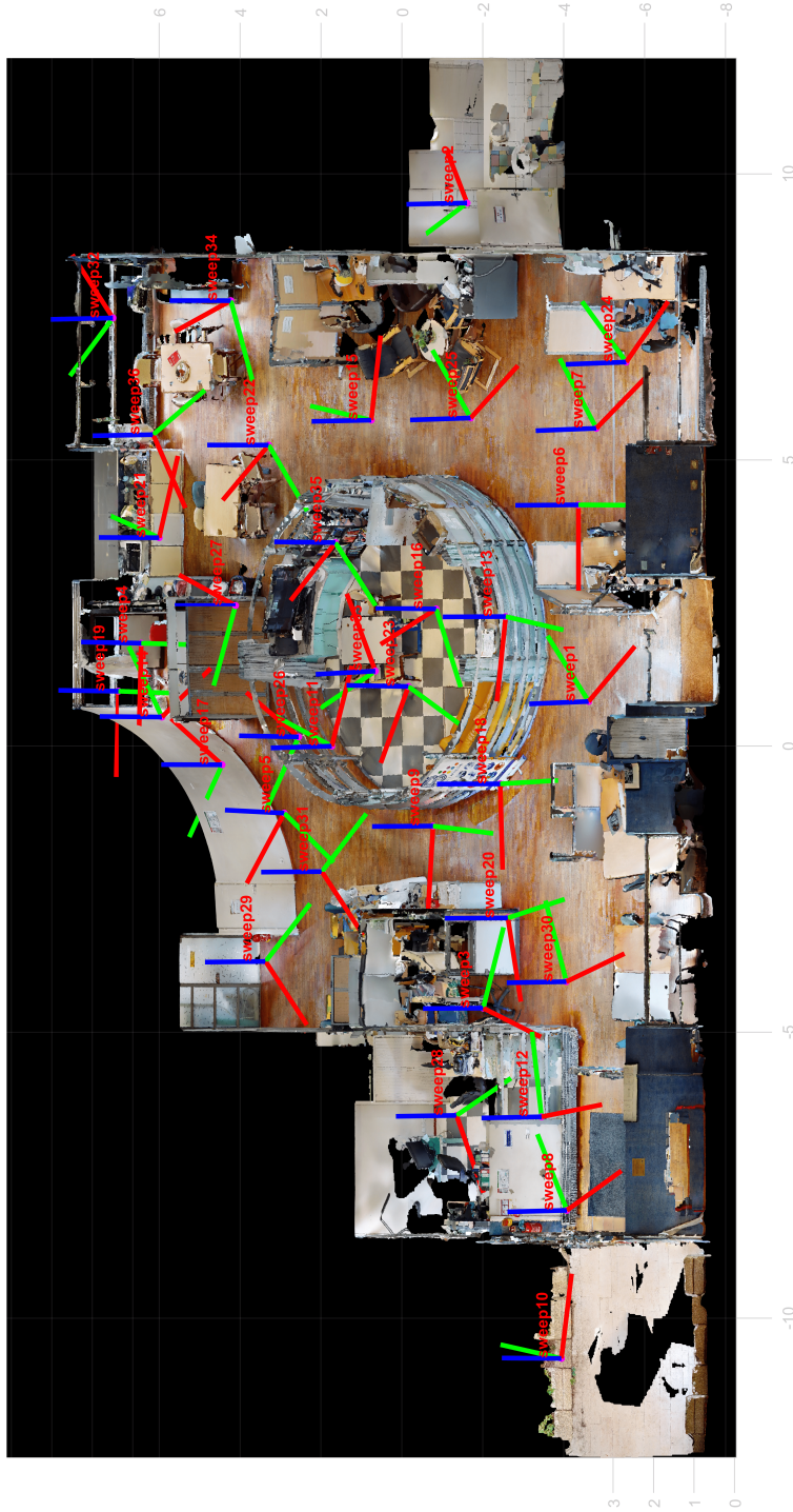
Figure 3.3: Coordinate systems of the sweeps are shown in the 3D map of the Living Lab scene.
