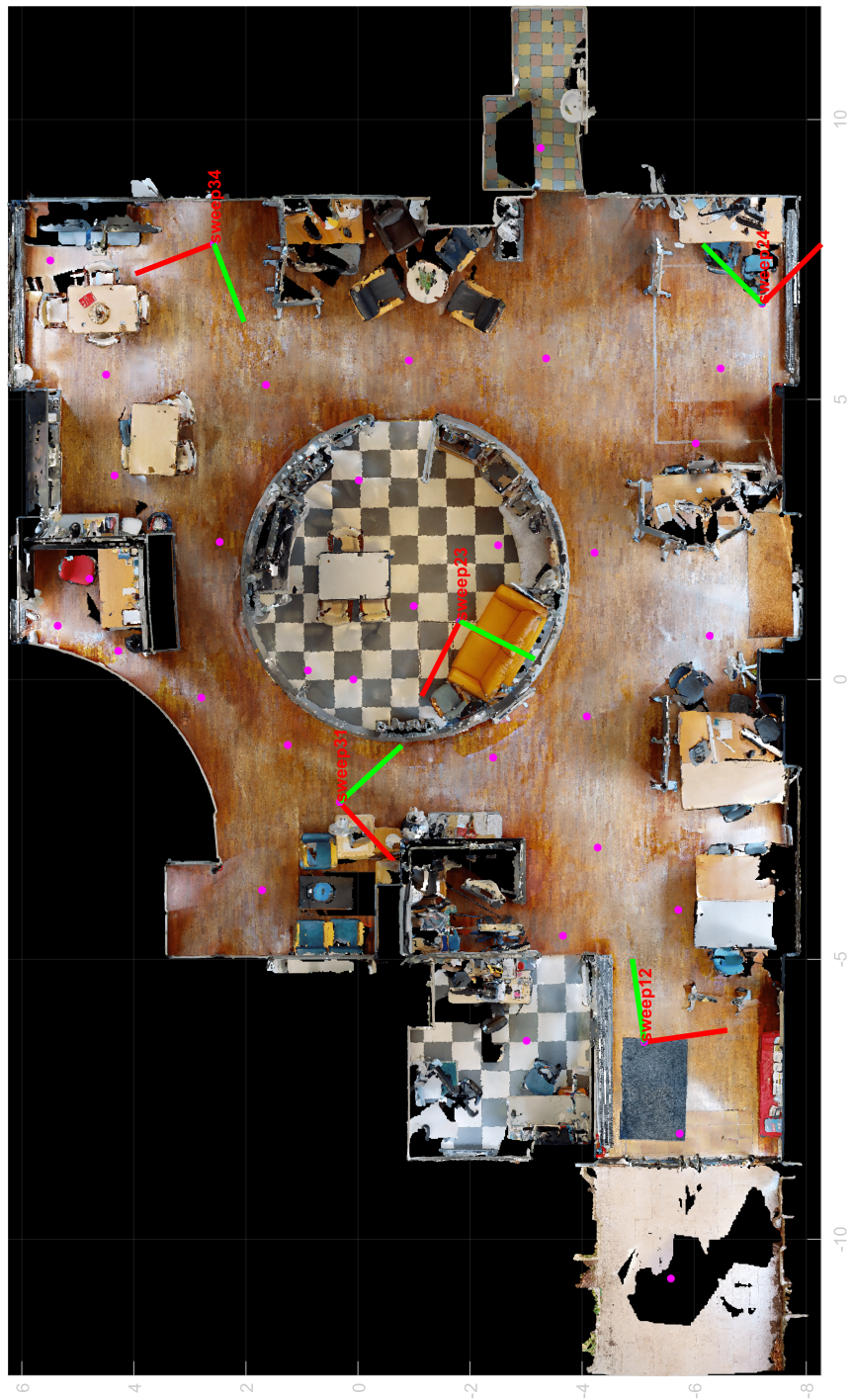
Figure 3.14: Living Lab scene with the locations of the coordinate systems of the sweeps that were used for queries. The pink dots are locations of the sweeps that were used for database images.
