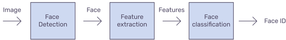
Figure 2.3: A face authentication pipeline [24]
