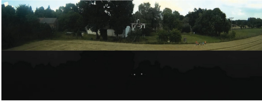
Figure 4.2: Comparison between the visible and UV camera footage from UVDAR, collected during an experiment. The UV image is significantly easier to process to retrieve information on the observed MAV [91, p. 2638].
