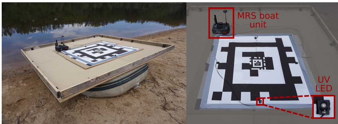
Figure 7.3: The USV with the landing platform used in real-world experiments.
