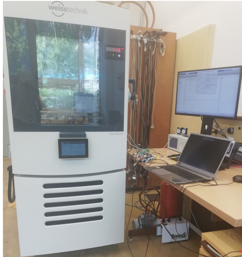
Figure 7.12: Laboratory setup with climatic chamber for the environmental test.
