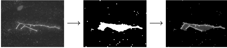
Figure 3.5: Example of thresholding a positive sample to obtain the binary mask, which is then used to extract the positive cutout for inpainting.
