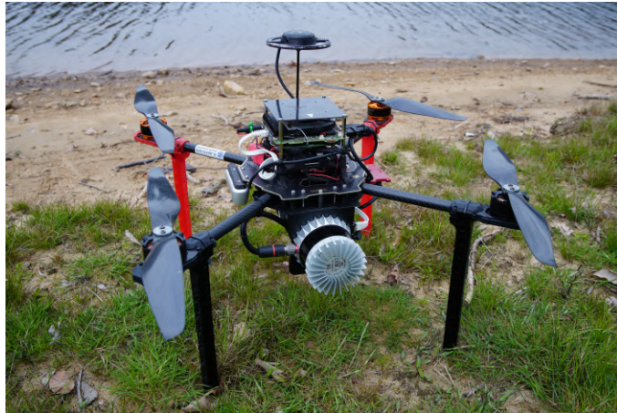
Figure 5.7: Image capturing lidar mounted on the UAV.
