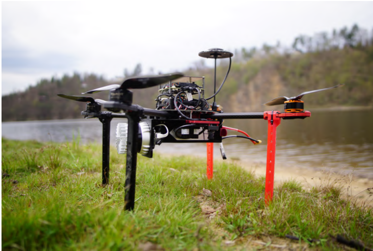
Figure 4.3: Image capturing Basler dart camera mounted on the UAV.
