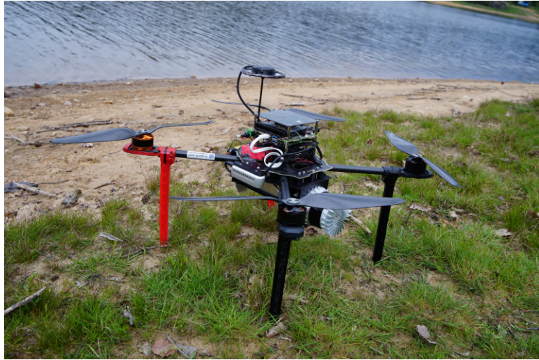
Figure 4.1: Image capturing Intel RealSense camera mounted on the UAV.
