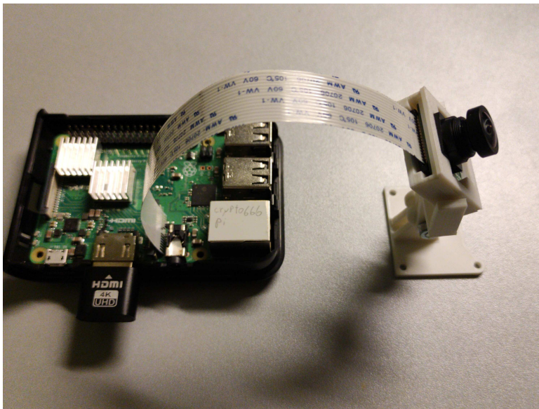
Figure 3.1: Raspberry Pi 3B+ and Camera module V2.1
