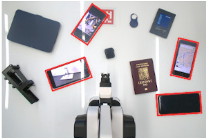
Figure 7.1: The touch screen device detection test setup. The non-phone objects from left to right are: the dropper, the Kindle, the Apple Watch, the access chip, the passport, and the computer drive.
