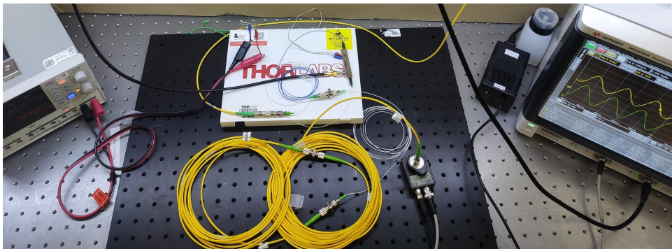
(b) : Photo off all components and devices, only signal generator and laser source are off the shot. Laser is connected to the intensity modulator. Optical fibres of which the length is measured follow. The end is connected to the photodiode. Electrical signal from the PD goes to the oscilloscope where the reference signal from signal generator is also shown.
