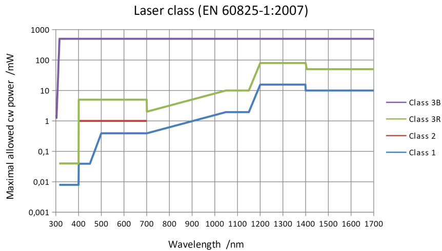
Figure 1.3: Maximal allowed continuous power for different wavelengths defined for different laser classes based on EN 60825 norm. From [9] (Created under Creative Commons license).
