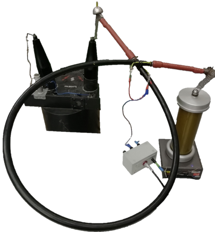
Figure 3.7: One of the tested cable termination specimens; the figure also depicts the test configuration employed in loss tangent measurements.
